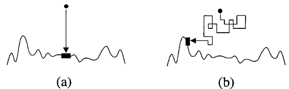
FIG. 1. Schematic diagram for comparison of the local noise (a) to the random-walk-like nonlocality (b) in erosion models. (a) The erosive process in the model with local noise occurs directly at a randomly chosen column as in ballistic erosion model. (b) The erosive process has more chance to occur at some protruded part of surface when a random walker mediates the process as in DLE model.
